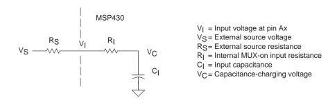
The resistance of the source  $R_S$  and  $R_I$  affect  $t_{sample}$ . The following equations can be used to calculate the minimum sampling time  $t_{sample}$  for a 10-bit conversion.
